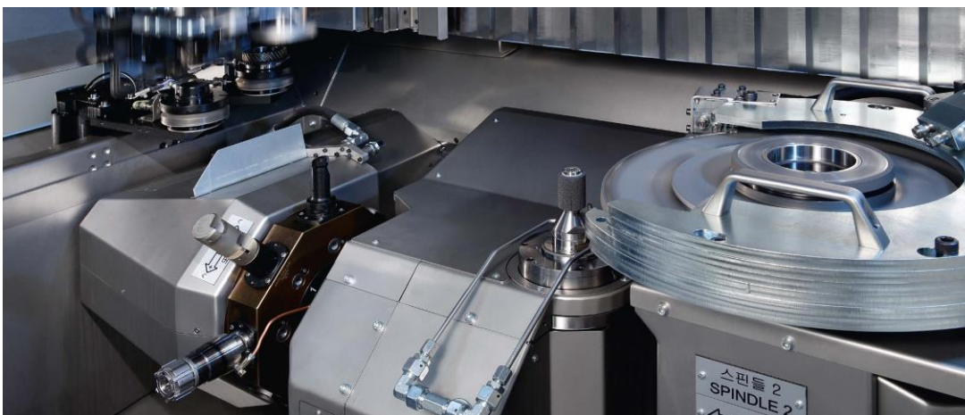
The working chamber with workpiece twin spindle
