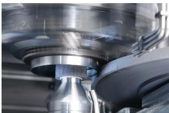
Simultaneous CBN grinding of cone and internal diameter
