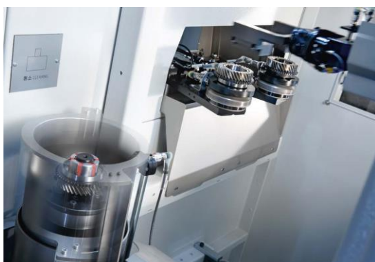
Loading device in the back and cleaning station in the front
